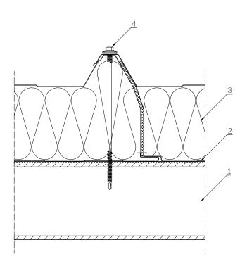
Select the tie according to the type and thickness of the underlying structure (steel, wood, reinforced concrete, etc.) The number of fasteners is specified in the characteristic loading tables.
