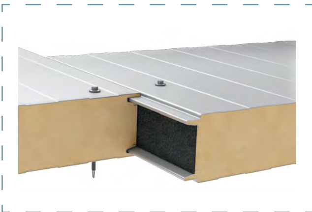
Panels connection scheme
