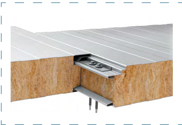
Panels connection scheme
