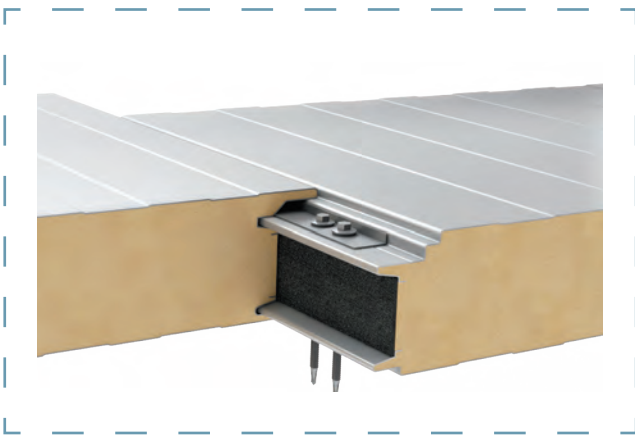
Panels connection scheme
