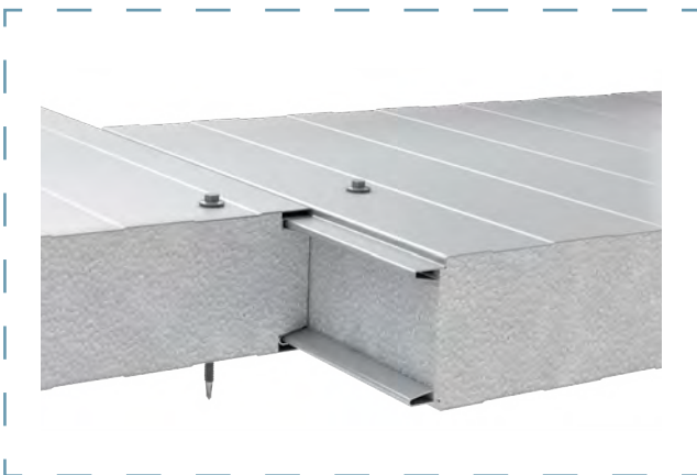
Panels connection scheme
